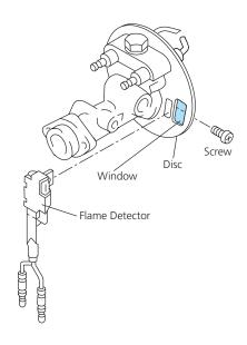
Figure 42: Flame Detector Replacement
