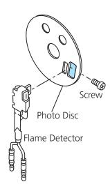
Figure 5: Flame Detector and Photo Disc
