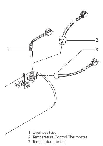
Figure 36: Temperature Control Elements
