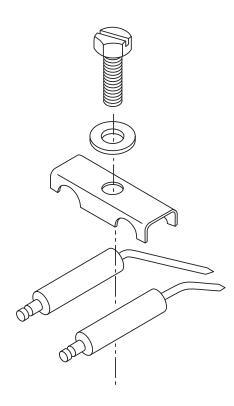
Figure 43: Ignition Electrode Replacement
