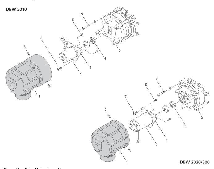
Figure 45: Drive Motor Assembly
