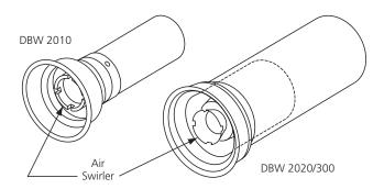
Figure 16: Combustion Chambers
