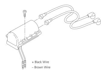
Figure 14: Electronic Ignition Unit
