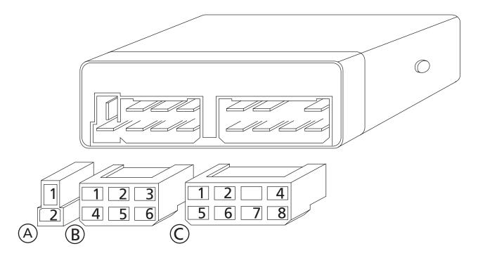
Figure 33: Control Unit - Identification of Terminals
