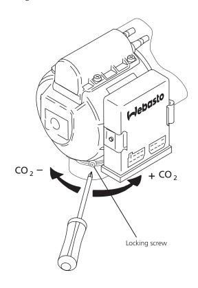
Figure 21: Combustion Air / Fuel Mixture Adjustment
