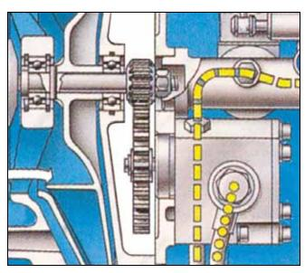
Figure 9: Fuel Pump Drive Gearing
