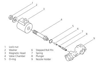
Figure 39: Fuel Valve and Solenoid Assembly
