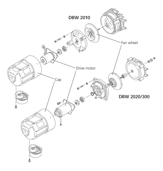
Figure 7: Combustion Air Fans
