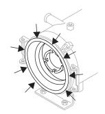
DBW 2010 burner tube removal. Carefully pry out with screw driver.
