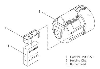
Figure 37: Control Unit Removal / Installation
