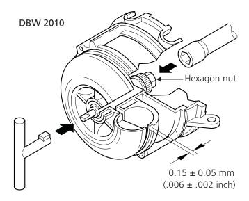
Figure 35: Clearance Adjustment - DBW 2010 Fan DBW 2020/300 ONLY:
