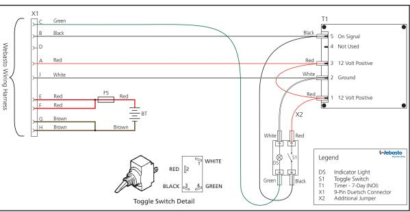
Wiring diagram - ISS Timer with optional Toggle Switch
