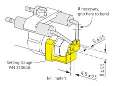
Figure 23: Setting of Ignition Electrodes
