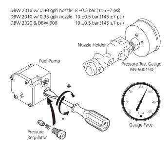
Figure 25: Fuel Pressure Check
