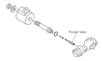
Figure 11: Fuel Solenoid Assembly
