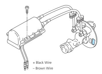
Figure 44: Ignition Coil Replacement
