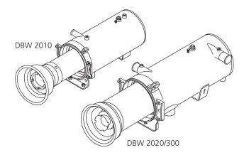
Figure 50: Burner tube replacement
