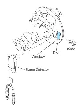
Figure 22: Flame Detector Check
