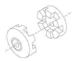
Figure 8: Motor to Fan Coupling (Clutch)
