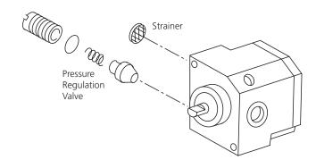
Figure 10: Fuel Pump Assembly
