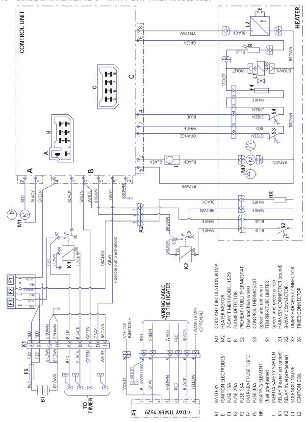
Figure 31: Schematic - Scholastic Heater™ With Digital 7-Day, 3 Program Timer Model 1529
