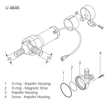
Figure 55: U4846 Circulation Pump - Exploded View
