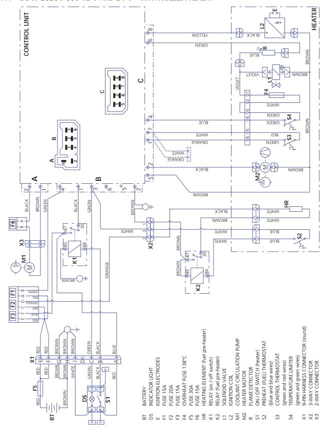
Figure 29: Schematic - DBW 2020 / 300 With Nozzle Preheat
