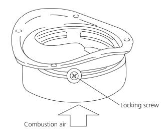
Figure 6: Combustion Air Intake Bellows
