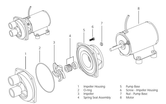
Figure 56: MP School Bus Circ. Pump - Exploded View
