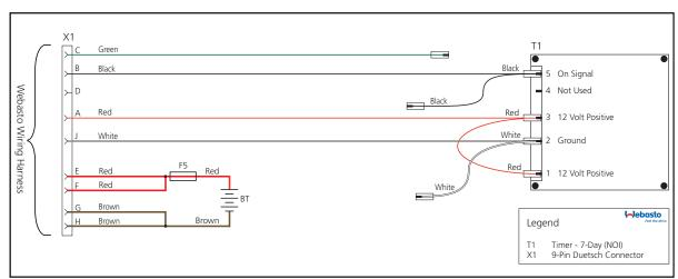
Wiring diagram - ISS Timer
