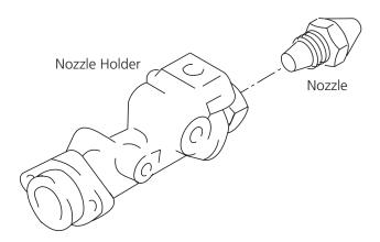
Figure 12: Nozzle Holder and Nozzle
